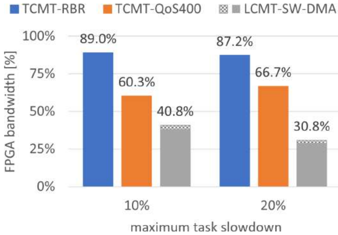
Fig. 13: Exploitation of the residual bandwidth from the FPGA-based accelerators. Average.
